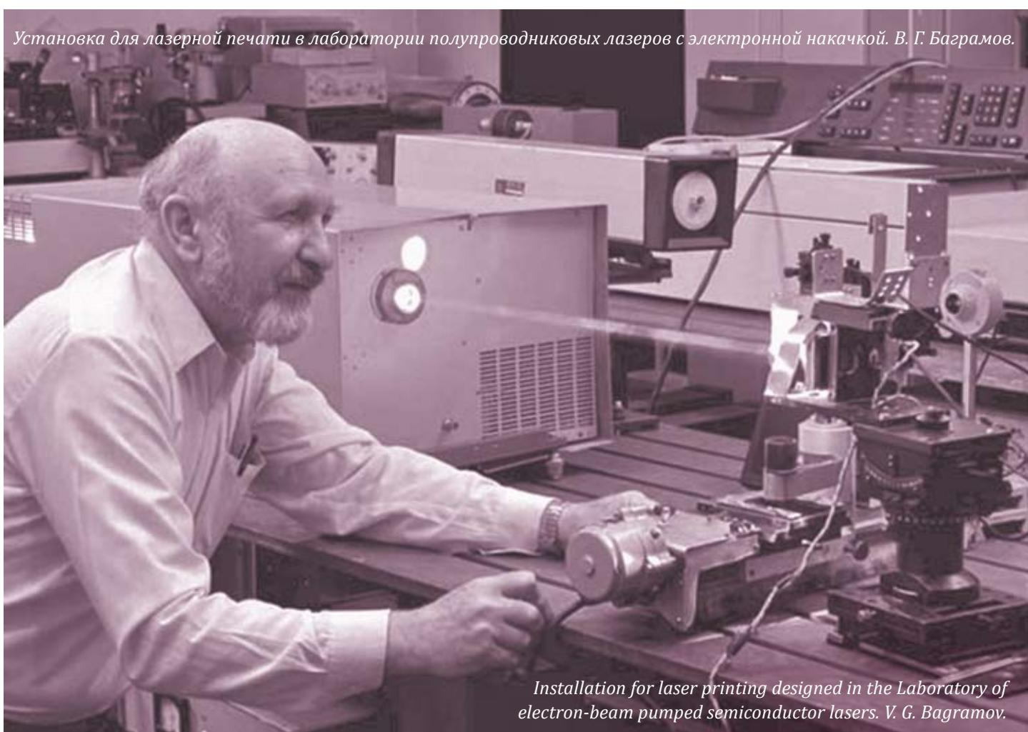
Installation for laser printing designed in the Laboratory of electron-beam pumped semiconductor lasers. V. G. Bagramov.
